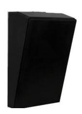
DB Sound PS12 is a high-end cinema surround speaker System, specially designed to reproduce high quality surround sound suitable for immersive sound playback. It is equipped with a full range 12" (31 cm) dual cone loudspeaker with a 90° conical horn. This surround system is tuned to obtain an extremely linear frequency response.
